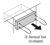
Note: Do not lose Removal Tools. They will be needed to remove the unit from the vehicle's dashboard.
